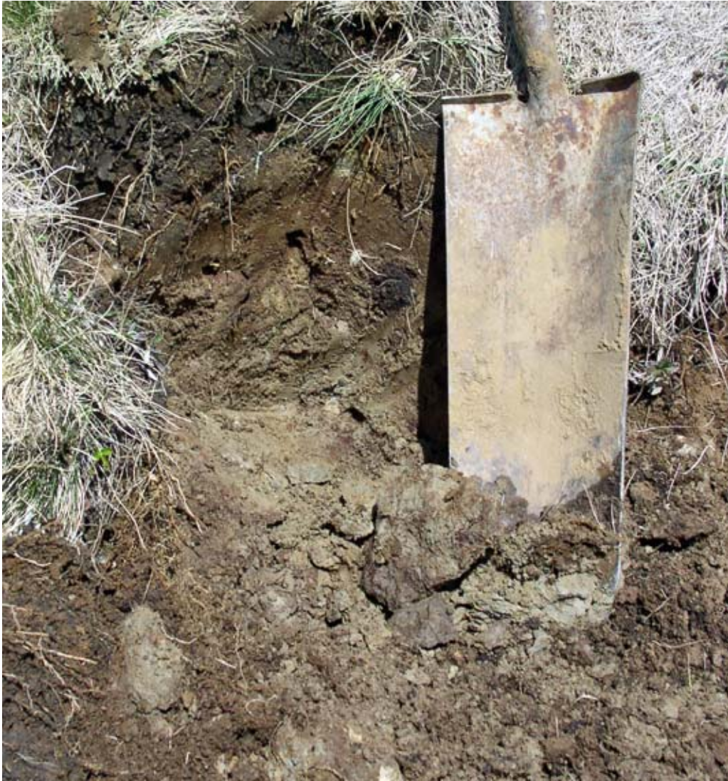
Figure 13.—An area of Crary-Adirondack complex, 0 to 8 percent slopes, very bouldery. The seasonal high water table in the Adirondack soil is perched at a depth of 0.5 to 1.5 feet. It is shown by the gray and brown mottles at the point of the sharpshooter (spade).
